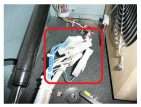
7- Remove the button panel assembly including the harness. Keeps for installation on the new belly door. You will install it at a later stage.
