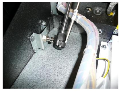
10-Using a 7/16" HEX socket, remove the urethane armrest from the original belly door assembly (three lock nuts).
