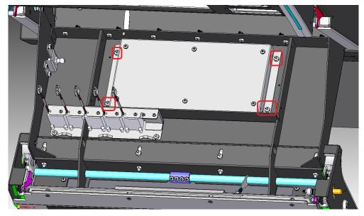
3- Remove (2x #8-32 lock nuts) mechanical meters assembly and keeps all parts and hardware's for installation on the new belly door. Disconnect meters from the button panel harness. You will install it at a later stage.
