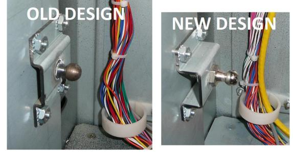
19-Install damper back into the cabinet. Simply push damper end fitting onto the ball joint until you feel a click. If damper has been broken, bent or do not properly operate, replace with a new one.
