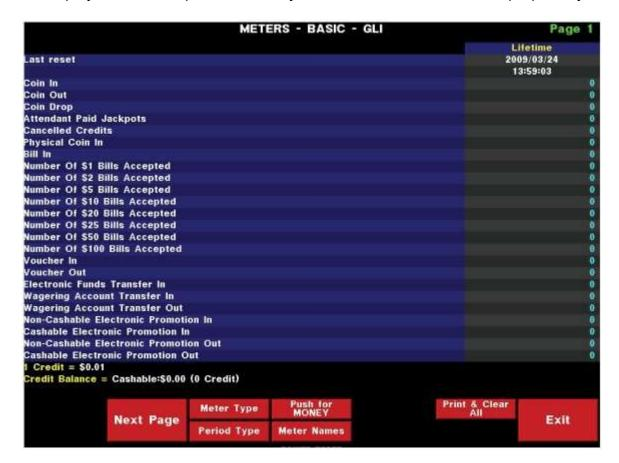
Last Reset indicates the date and time of the last mechanical-meter manual reset.
