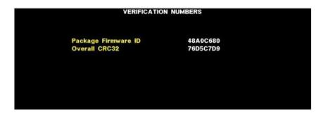
**Package Firmware ID** The unique identification number of the current software version. **Overall CRC32** The CRC 32-bit computation (Cyclic Redundancy Check) performed on the downloaded software.
