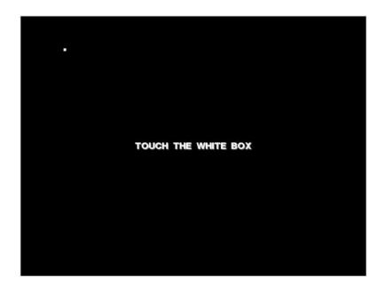
The calibration screen can be directly accessed by turning the Clear Error key while powering on the gaming machine. Hold the key until the calibration screen appears. This may take a few seconds.
