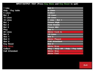
The gaming-machine inputs are listed in the left column. Asterisks identify the inputs already tested while red characters identify inputs currently being tested. Outputs are listed in the right column. To test an output represented by a red box, turn the Operator Menu key while pressing the box.
