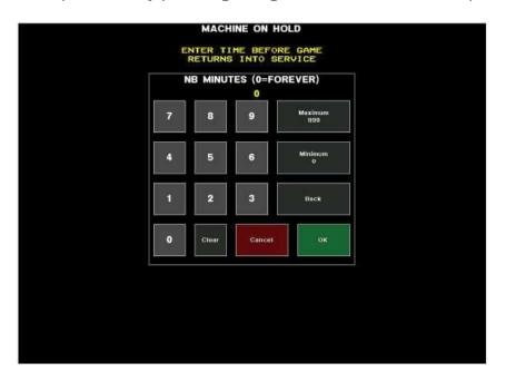
Using the numeric keypad, set the machine holding period. The maximum value allowed on the keypad is 999 minutes, but entering 0 allows the machine to be put on hold indefinitely This screen is displayed once the Player Hold option has been activated:
