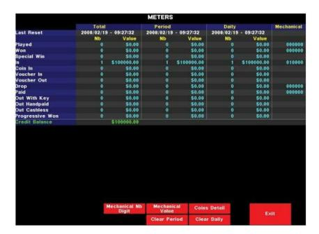
**Last Reset** indicates the date and time of the last mechanical-meter manual reset using the MECHANICAL VALUE button.
