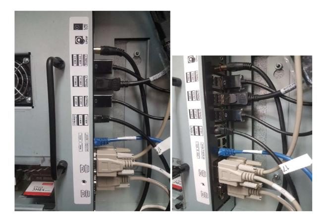
Most of the cables are labelled so that they can be easily identified and placed into the proper socket.
