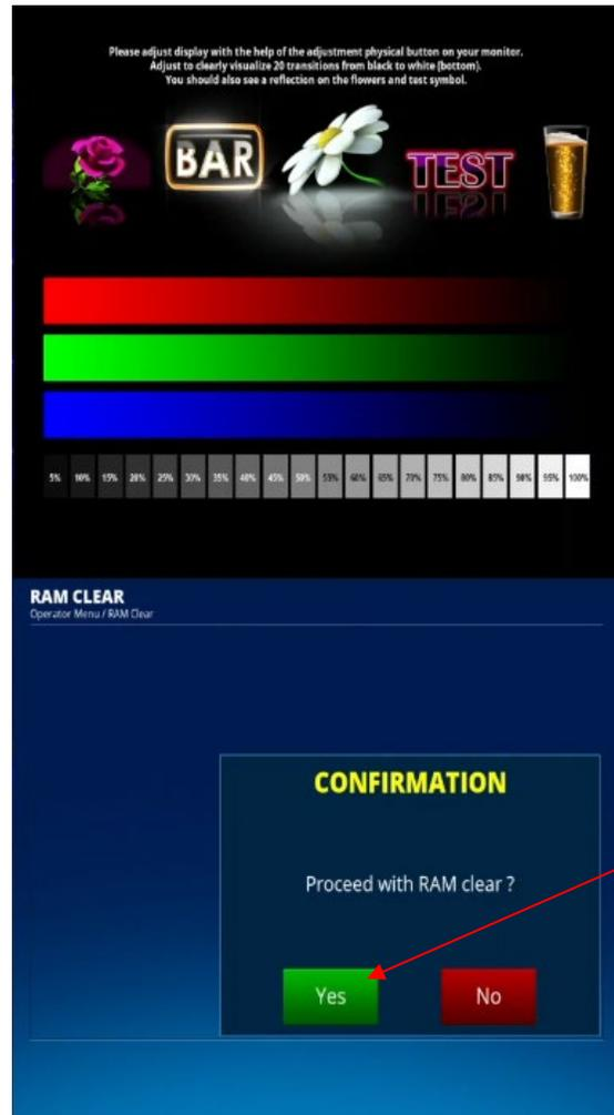
Once the process completes and 'Done' appears on the screen, power down the EGM and remove the RAM clear CF card.
