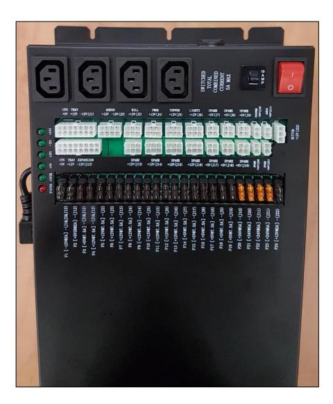
Each component inside the cabinet is powered independently from the power distribution unit. Each segment is fuse protected. To quickly determine whether a fuse is blown, check the LED under it.
