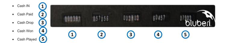
These meters, which cannot be reset, confirm data contained in the gaming board memory. They increment each time a 12 VDC pulse is registered. The hard meters are visible underneath the deck panel.
