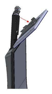
Rest the topper sideways on top of the main monitor, securing it with one hand. With your other hand, unplug the topper's power, DisplayPort, and Digi-Hub USB-B cables.
