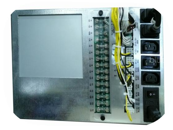
Each component inside the cabinet is powered independently from the power distribution unit. Each segment is fuse-protected. To quickly determine whether a fuse is blown, check the LED under it.
