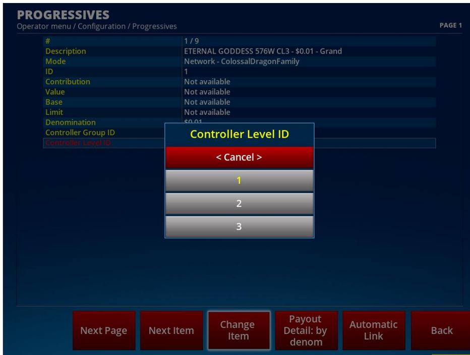
Figure 25: Set controller level.
