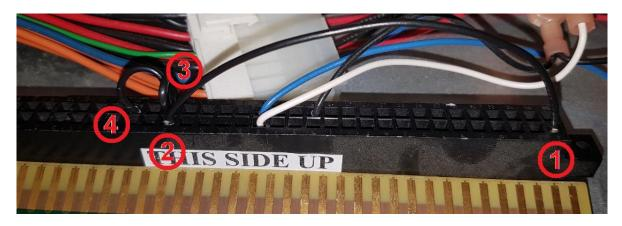
→ Build an harness as shown below for the logic door switch. Fast disconnect and crimps are included with the kit.
