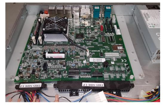
→ Install the Spider board inside the progressive controller box as shown.
