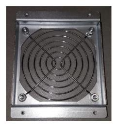
→ Attach the fan assembly and CFAST card cover to the progressive box cover using 6pcs #4-40 x 3/16 pan head screws.
