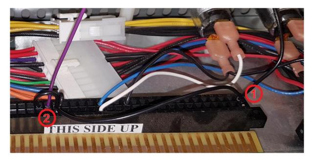
→ Install the ground wire (black) onto the switch (COM) before you insert the switch inside the holding bracket.
